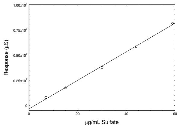
Figure 3.5.2. Calibration curve of sulfate. ( $Y = 141486X - 332515$ )
