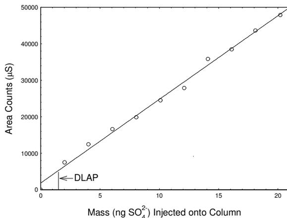
Figure 4.1. Plot of data to determine the DLAP. (Y = 2293X + 1839)
